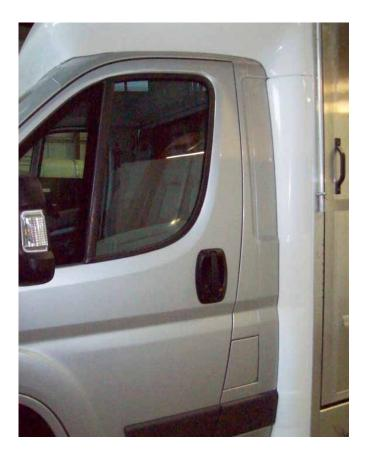
Once the horsebox is built it can be difficult to spot the difference. However, if there is almost no space between the cab door and the 'cuff' where the body begins then it is probably a 'cut & shunt'. If there is a good distance as shown in the photo below, it is probably built on a chassis cab.
